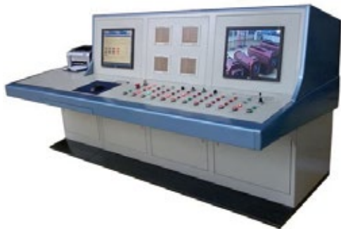
COMPREHENSIVE EXPERIMENTAL PLATFORM FOR POWER TRANSFORMER
